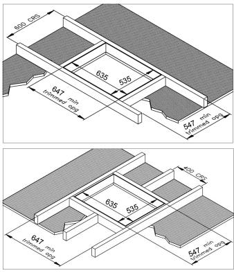
The AH6 is supplied with a safety wire secured to the lid. Place the loop of the wire between frame and Supalux in line with the middle fixing hole and secure with screw supplies. Fix the rest of the frame to the joist using 55mm long stainless steel screws through the remaining holes in the frame, ensuring that the frame is pushed tight against the ceiling to compress the foam seal. Finally replace the temporary nails with screws.
